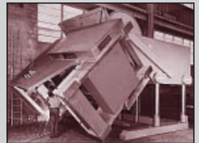
Floor level welding at capacities up to 350,000 pounds is easily achieved with Koike Aronson's Geared Elevation
