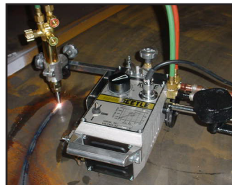
Circle cutting option cuts circles from 38-2450mm (1 1/2 - 96in) in diameter.
