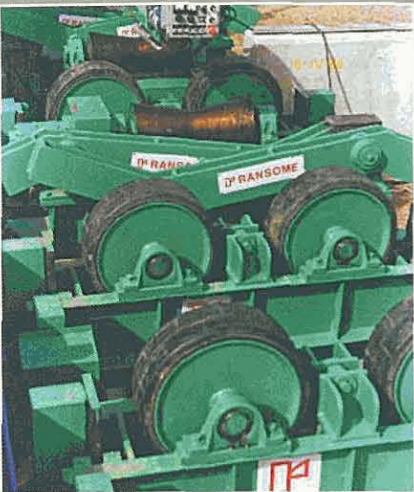
Elevating turning rolls for brace rack welding line.
