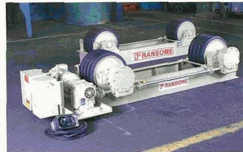
Ransome Power and Idler Roll diameters, centers and heights are designed for interchangeability among Models A, AA, AAA and among Models B, C, D and E.
