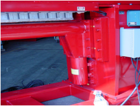
Cantilevered mandrel arm
