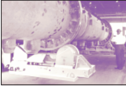
The Koike Aronson 600 Tonner Driver and Idler Turning Rolls shown positioning a Steam Drum.
