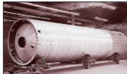
Trac-Tred turning rolls insure the most delicate care for thin walled vessels.
