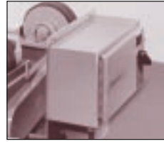
NEMA-12 Dust Tight Electricals.
