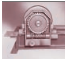
All-Steel Gearcase Final Drive is completely enclosed with lifetime lubrication.
