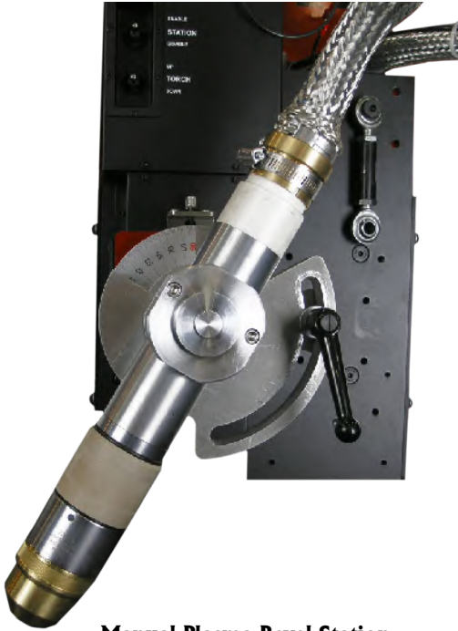
Manual Plasma Bevel Station Bevel in the rail axis only. Non-contour mechanical adjustment from +/- 0 - 45°.
