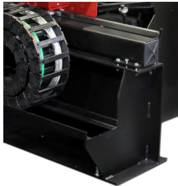
Rail Axis Drive Rail Precision ground rail and rigid pedestal weldment provides the stability for smooth and accurate machine motion.
