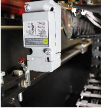
Rail Axis & Cross Axis Limit Switches Used for over-travel as well as homing of the machine.
