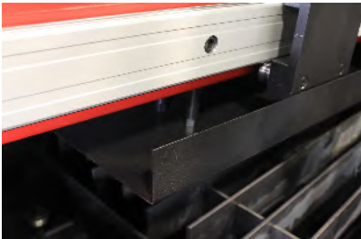
Linear Way and Heat Shields Replaceable linear roundway provides for a smooth and accurate cutting motion. Heavy duty heat shields protect machine from heat and sparks.
