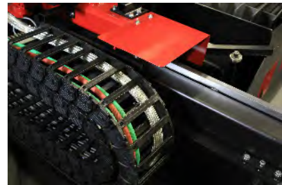
Rail Axis Cable Carrier Is mounted to the rail pedestal weldment. The cable carrier keeps all of the hoses & cables organized during machine movement.
