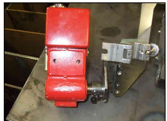
Remove WU-1 and use opposite Holes to remount on slide assembly
