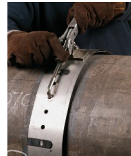
Adjusting Chain Links for Various Diameters
