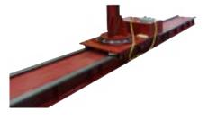
Powered and manual travel cars can be used for long seam welding or moving a manipulator from seam to seam.
