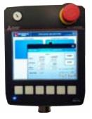
The independent hand held touch screen Human Machine Interface (HMI) communicates with VFD drive on the positioner, and provides real-time display of linear speed for the reach axis. Additionally, the HMI can command the linear speed target, either user set or on the fly adjustment.
