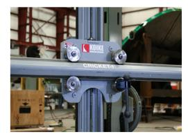
**Powered Vertical Lift** Ball screw driven lift for smooth operation, 20 IPM constant speed lift with pendant included.
