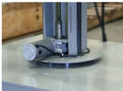
Manual Mast Rotation A graduated bevel collar ensures accurate bevel setting.
