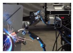
Pipe Welding Package Includes Wel-Handy Next Programmable WU-3 Weaver and control 3 in x 3 in manual cross slide Mounting brackets for pendants and welding controls
