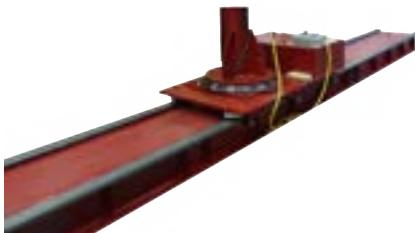
Powered and manual travel cars can be used for long seam welding or moving a manipulator from seam to seam.
