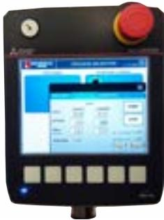
The independent hand held touch screen Human Machine Interface (HMI) communicates with VFD drive on the positioner, and provides real-time display of linear speed for the reach axis. Additionally, the HMI can command the linear speed target, either user set or on the fly adjustment.
