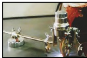
Large circle compass \varnothing 5-19 ¾ in (ø125- 500mm) Part#ZS30106
