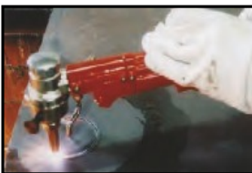
Attachment for small circle cutting \varnothing 1¼-8 in (ø30- 200mm) Part#61001597
