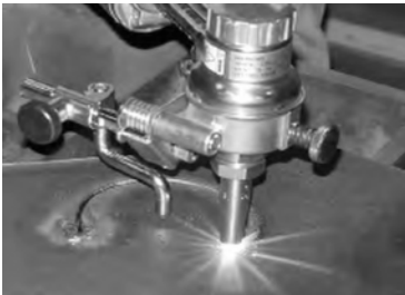
Small circle cutting attachment 1¼ to 4½ in (30-120mm) (Included in all kits)
