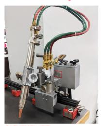
**OXY-FUEL KIT**Cut up to 10" thick material.
