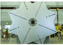
**Flex Plate Fixturing Table** Offers flexible machine connection to protect against misalignment and thermal expansion alignment issues.
