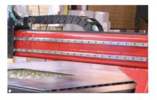
Heavy-duty Linear Bearings both "X" & "Y" Axis
