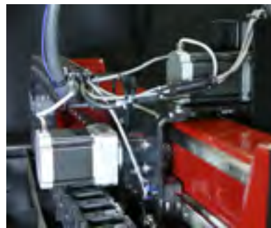
Precision Low Backlash Gearboxes Large 25mm linear bearing on short axis and 30mm bearing on the cross for smooth motion
