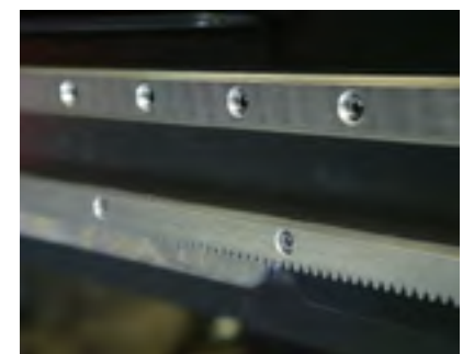
Helical Gear Rack with AGMA 12 grade ground pinions
