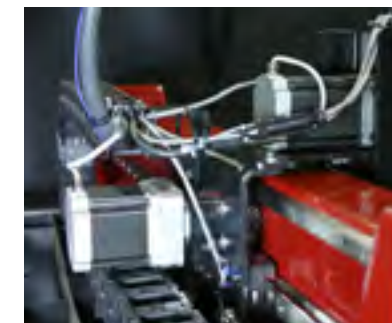
Precision Low Backlash Gearboxes Large 25mm linear bearing on short axis and 30mm bearing on the cross for smooth motion
