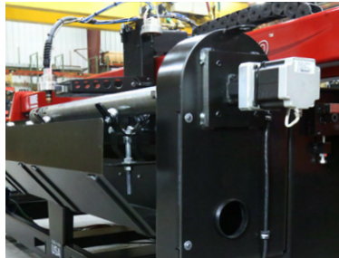
THROUGH-HOLE CHUCK DESIGN WITH BUILT-IN SPARK ARRESTOR
