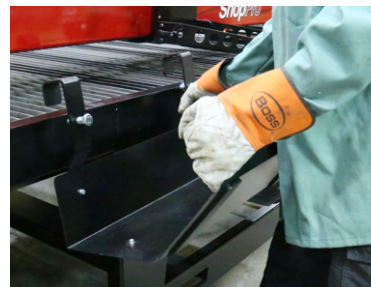
REMOVABLE SLAG PANS FOR EASY CLEAN UP
