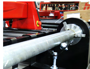
THROUGH-HOLE CHUCK DESIGN WITH BUILT-IN SPARK ARRESTOR
