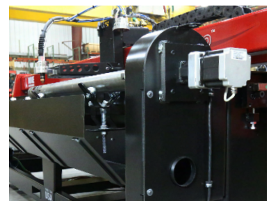
THROUGH-HOLE CHUCK DESIGN WITH BUILT-IN SPARK ARRESTOR
