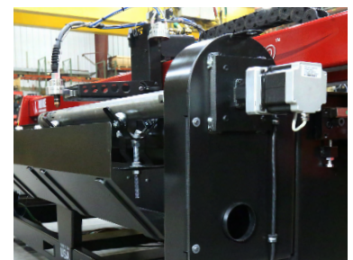
THROUGH-HOLE CHUCK DESIGN WITH BUILT-IN SPARK ARRESTOR
