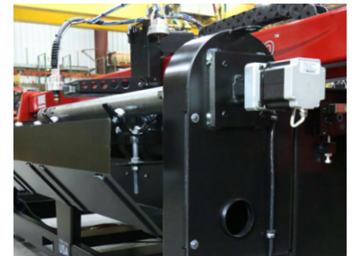
THROUGH-HOLE CHUCK DESIGN WITH BUILT-IN SPARK ARRESTOR
