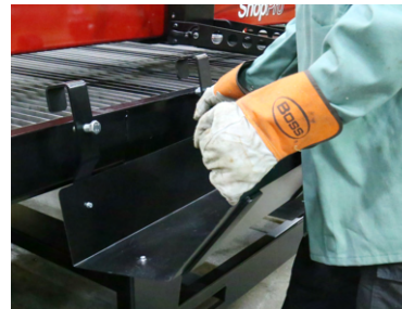
REMOVABLE SLAG PANS FOR EASY CLEAN UP
