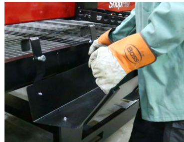
REMOVABLE SLAG PANS FOR EASY CLEAN UP
