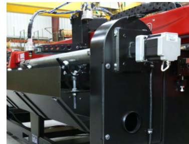
THROUGH-HOLE CHUCK DESIGN WITH BUILT-IN SPARK ARRESTOR
