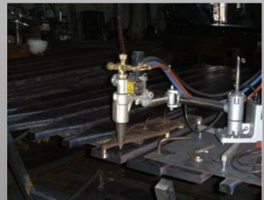
**Easy Tip Replacement:** The tip can be easily cleaned and replaced. Flame adjustment is made easy by simply raising the tracer head.
