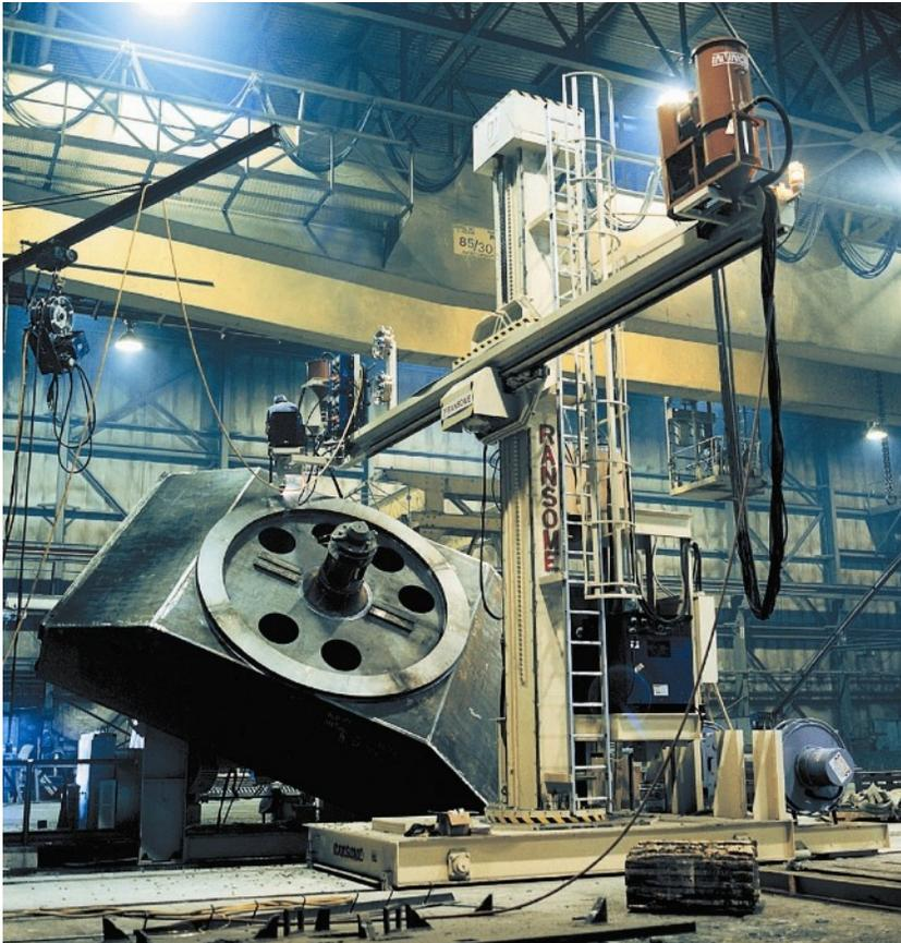
The Koike Aronson/Ransome large range chain lift manipulators can be customized for specific applications, such as simple straight-line to circumferential welding. The Ram ends can be outfitted with small I.D. single or multiple arc welding heads for long seam and circumferential welding procedures. We have custom designs that can handle extra heavy, and extra long reach applications.
