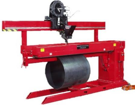
The fixed height mandrel is incorporated into the machine base with provision to attach gas purge and water cooling capability if necessary, water cooling requires an in-house water supply or water chiller with pump. A replaceable copper backing bar is attached to the top of the mandrel. Retractable alignment mechanisms are provided for aligning the plate.
