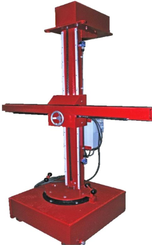
Koike Aronson / Ransome model 44 manipulator is perfect for small open arc welding applications. A manual rack and pinion reach gives the operator precise control for positioning the arc. The powered reach axis allows for quick height adjustment and for carrying to a maximum of a 300 lb load that the ram can carry. Manual mast rotation allows the entire machine to be rotated and repositioned over multiple stations.
