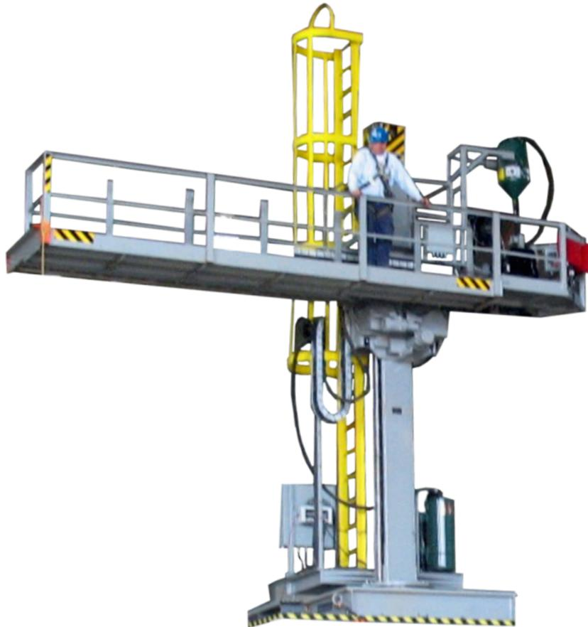
Koike Aronson / Ransome gear elevated Scarab series Manipulators are designed for safety and a trouble free long life. All critical mechanisms are enclosed and load carrying gear cases are welded in place and lifetime lubricated. Both lift and reach axis are guided with concave wheels and roundways for precision movement.
