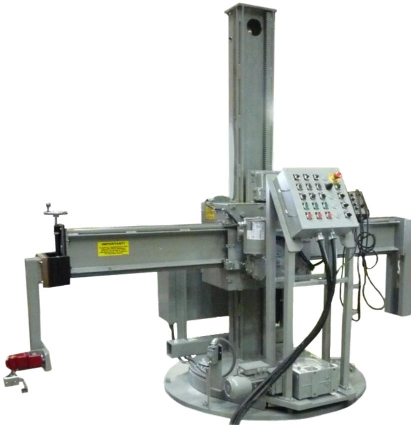
Koike Aronson / Ransome gear elevated Locust series manipulators are designed for safety and a trouble free long life. All critical mechanisms are enclosed and load carrying gear cases are welded in place and lifetime lubricated. Both lift and reach axis are guided with concave wheels and roundways for precision movement.
